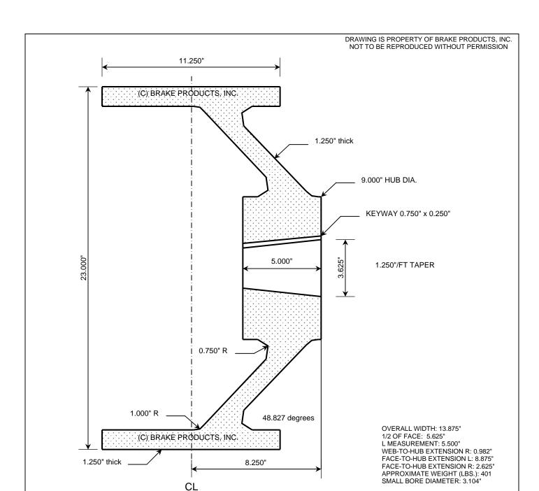
TOLERANCES: WHEEL DIAMETER: +0.005"/-0.000" BORE TAPER: +0.000"/-0.003"
